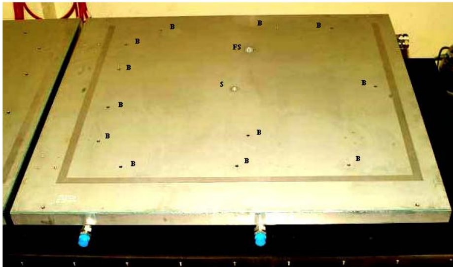
Stbd Flight BPA B: EVA Bolt Interface S: Shear Pin Interface FS: Floating Pin Interface
