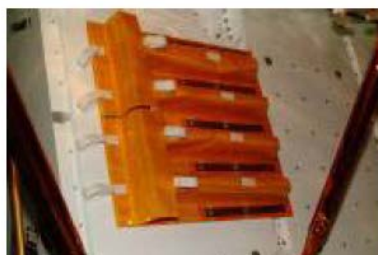
Figure 3-67. Large and small MLI contingency stowage pouches
