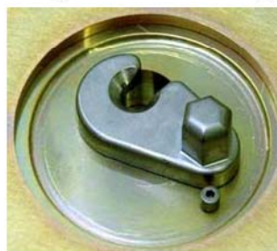
J-Hook Assembly installed to the Base Plate
