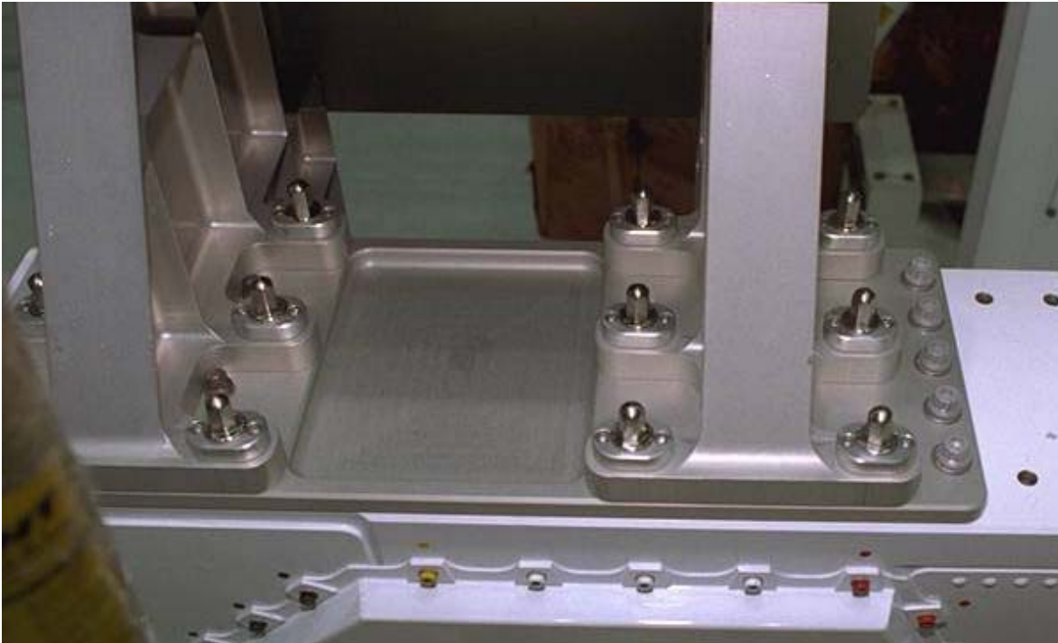
Figure 3-43. Forward fixture EVA bolts
