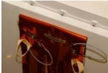
Figure 3-68. MLI tool storage sheath
